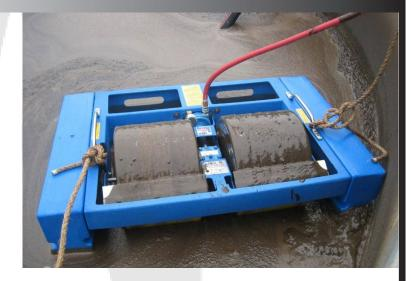
recover oil at rates up to 20 gallons min/ 5 cu.m per hour. The self-adjusting wiper blades recover oil from the face of drums as they rotate. SKIMOIL DrumSkimmers are able to recover a wide range of oils and sheen, from diesel to crude oils. The motor, gearbox and drums are capable of thousands of hours of trouble free operations. SteelMAX may be fitted with either an air or hydraulic drive. We offer a choice of suction pumps in different material to suit the application.
